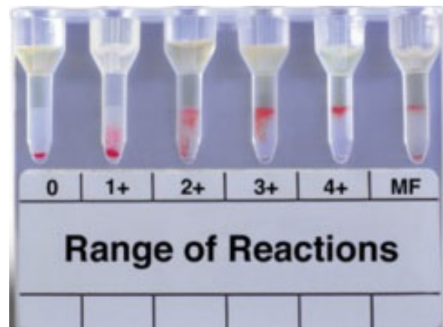
Fig 1 — Grading of DAT reaction (Taken from Card Instruction Manual of Micro Typing System MTS084024 Anti-Human Globulin Anti-IgG MTS Anti-IgG)
